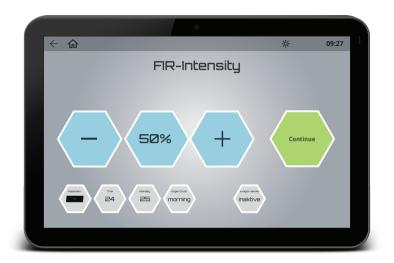
If you have a whole body infrared mat (Exagon FIR), you can use the hybrid option to start a magnetic field application with integrated infrared application. The setting parameters are expanded by the option to define the temperature intensity of the infrared whole body mat.
