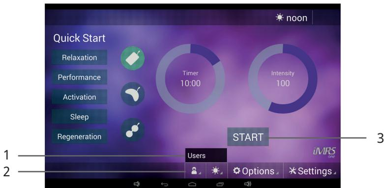
Connect the D/A converter 2.0 and the desired applicator (see Chapter 13, Installation) and start the Omnium1 2.0 application (see Chapter 14, Activation). After the system has been successfully started, chose the desired application duration. To do so, tap the circle next to Timer (1) and set the desired application duration from 1 to 60 minutes. It can be set in steps of 1 minute.
