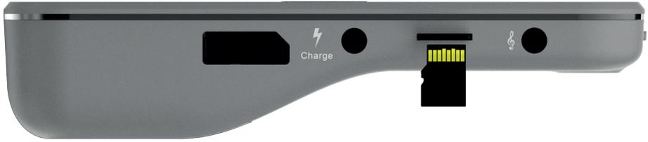
Insert a micro SD memory card (max. 32 GB) in the card slot as shown in the picture of the device. Do not push hard or use any force. The card only needs to overcome a light spring resistance. Once the memory card is properly positioned, it will lock into place instead of being ejected.
